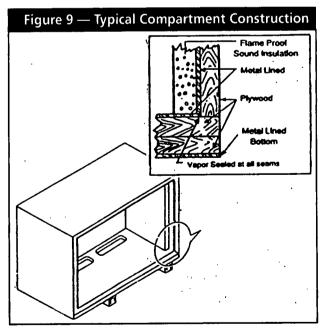
• Line the entire compartment interior with 26 gauge galvanized steel as described above.
